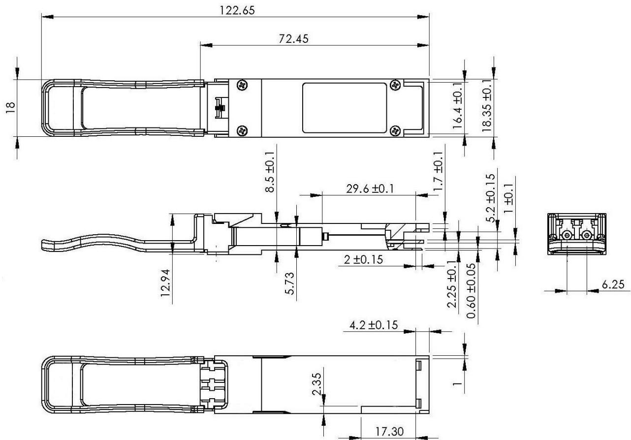
(All Dimensions are  $\pm 0.20\text{mm}$  Unless Otherwise Specified, Unit: mm)
